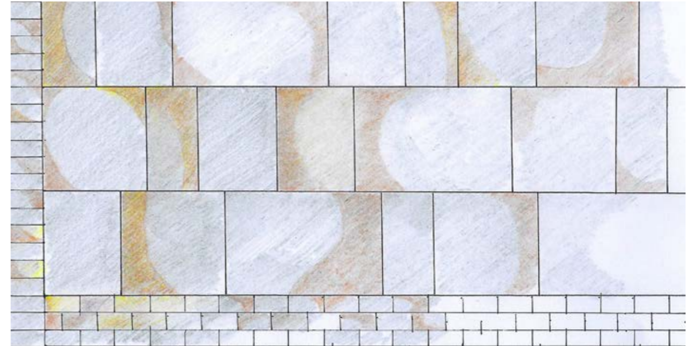
As shown above the application of stone pavers in random lengths gives an irregular pattern that feels softer and more inviting, while supporting the prolonged availability of finite materials.
